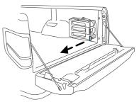
2. Open the latches to release the panels.
