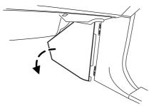
To remove the fuse box cover, press in the tabs on both sides of the cover, then pull the cover off.
