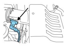
2. Reposition the locking clip on the connector (connector shown from below for clarity), squeeze the connector and pull it off of the air outlet tube.
