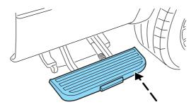
To stow the box side step, with your foot, push the box side step under the truck until fully latched. Do not push on the button while stowing the box side step.
