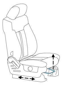
Pull the release lever handle located on the side of the seat up to move the seatback forward or backward.
