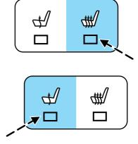
The heated seat module resets at every ignition run cycle. While the ignition is in the on position, activating the high or low heated seat switch enables heating mode. When activated, they will turn off automatically when the engine is turned off.
