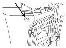
3. Loosen the three retaining bolts (two at top of lamp, one at lower inboard corner).
