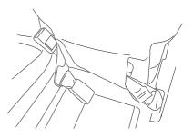
Before a passenger sits in the front center seat, make sure the lap belt and buckle are both placed in their in-use position, and no longer stowed. Always fasten your seat belt when riding in the front center seat.
