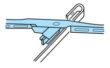
Replace wiper blades at least once per year for optimum performance. Poor wiper quality can be improved by cleaning the wiper blades and the windshield. Refer to *Windows and wiper blades* in the *Cleaning* chapter.
