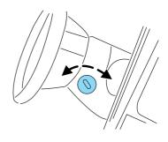
4. Turn the hazard flashers on then off three times. This must be accomplished within 10 seconds.
