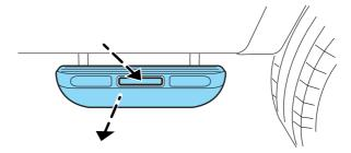
To deploy the box side step, with your foot, push down on the button. The step will automatically extend out from the stowed position.
