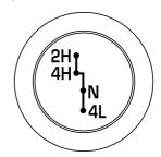
**4L (4X4 Low)** – Uses extra gearing to provide maximum power to all four wheels at reduced speeds. Intended only for off-road applications such as deep sand, steep grades or pulling heavy objects. The shift lever will not engage 4L (4X4 LOW) until the transmission is in N (neutral) and the vehicle is moving below 3 mph (5 km/h); this is normal and should be no reason for concern. Refer to *Shifting to/from 4L (4X4 Low)* for proper operation.
