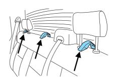
and as an anchoring loop for child seats installed in the outboard rear seats.
