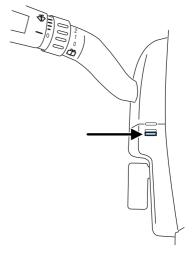
4. Insert a flat head screwdriver into each slot to unsnap and remove the steering column cover. Rotate the column up on its hinges and pull rearward to remove the cover from the hinges.
