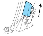
5. With the ignition in the on position, pull back on the BSI solenoid found on top of the uncovered steering column and at the same time, apply the brake pedal and shift the transmission into N (Neutral).
