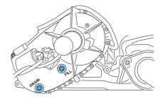
3. Add only enough fluid through the filler opening so that the fluid level is at the bottom of the opening.
