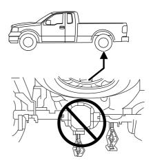
**WARNING:** To lessen the risk of personal injury, do not put any part of your body under the vehicle while changing a tire. Do not start the engine when your vehicle is on the jack. The jack is only meant for changing the tire.
