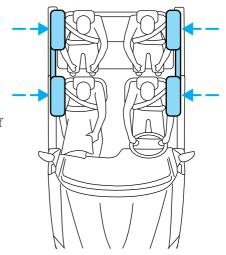
The safety canopy is mounted to roof side-rail sheet metal, behind the headliner, above each row of seats. The safety canopy is designed to inflate between the side window area and occupants to further enhance protection provided in side impact collisions and rollover events.
