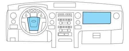
The airbag supplemental restraint system is designed to work in conjunction with the safety belts to help protect the driver and front outboard passenger from certain upper body injuries. The term "supplemental restraint" means the airbags are intended as a supplement to the safety belts. Airbags alone cannot protect as well as airbags plus safety belts in impacts for which the airbags are designed to deploy, and airbags do not offer any protection in crashes for which they do not deploy.
