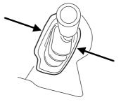
3. Turn the steering wheel one-half turn to access the slots on each side of the steering wheel.
