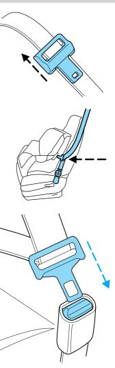
6. While pushing down with your knee on the child seat pull up on the shoulder belt portion to tighten the lap belt portion of the combination lap and shoulder belt.
