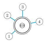
3 (on) position. The locks will cycle to confirm that the programming mode has been entered.
