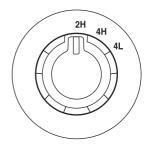
**4L (4X4 Low)** - Uses extra gearing to provide maximum power to all
