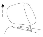
3. Lower the head restraint by pressing and holding the guide sleeve adjust/release button and pushing down on the head restraint.
